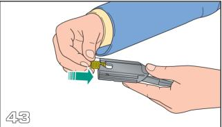
4) Slide the bolt head into the bolt carrer, making sure that the hole on its shaft coincides with the slot on the bolt(fig.44)
