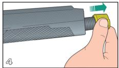
For models equipped with short tube magazine plus magazine tube extension (magazine tube in two pieces), the extended magazine tube is coming off together when unscrewing the forearm cap. NOTE: Before proceeding, you must read and follow the instructions "Magazine tube extension"
