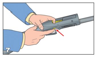
5) Install the forearm on the barrel. The forearm must first be slid over the barrel guide ring (fig. 8) and then snapped onto the barrel (fig. 9).
