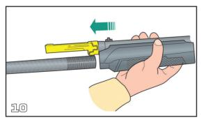
7) As the barrel extension nears the bolt group, carefully align the barrel hood with the top of the protruding bolt head.
