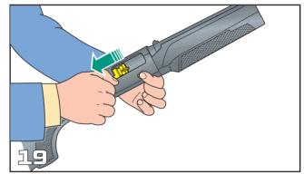
2) With the bolt closed and the hammer cocked, roll the gun with the magazine port up and pointing the barrel downwards.
