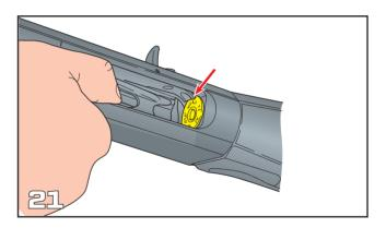
NOTE: The gun must be loaded with the hammer cocked so that the magazine latch can retain the cartridges as they are inserted in the magazine. Now the gun cannot be fired unless a cartridge is placed in the barrel, following the procedure:
