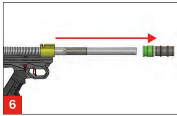
You can remove the dual gas system and gas piston by sliding to the arrow and clean or maintenance your gun.
