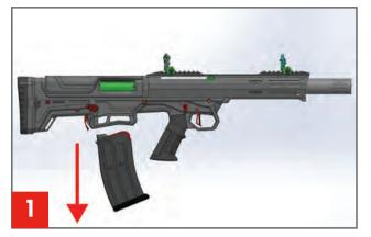
Push the magazine release button and remove the magazine from gun.
