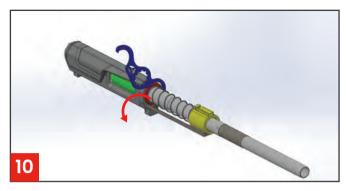
Turn barrel nut to anticlockwise with the latch wrench in your box for removing the barrel not as shown in the diagram.
