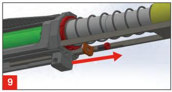
Turn barrel fixer nut screw by T15 wrench to anticlockwise ,then remove the screw and barrel nut fixer latch as shown in the diagram.
