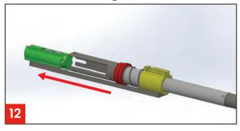
Pull back the bolt carrier as on the diagram for removing the bolt body.
