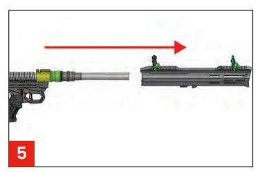
Handguard of your HURACAN GT12 can now be removed easily by sliding it forward.Now your HURACAN GT12 will be ready for cleaning of the gas system and mechanical areas.
