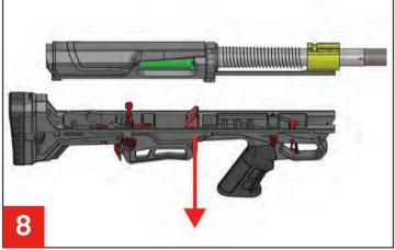
We do not suggest to disassemble your upper if it is not a need for your guns performance. If you need to do field maintenance for your gun you can pull the takedown pins back and seperate upper and lower frame of your gun.
