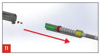
You can slide barrel group assembly easily to arrow direction now.
