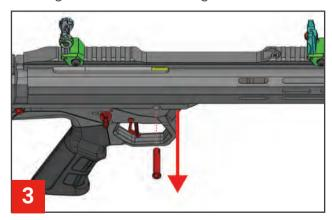
Pull the rear takedown pin to direction of the arrow as shown in the figure.
