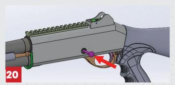
20- Insert the fire control group retaining pin.(fig. 20)
