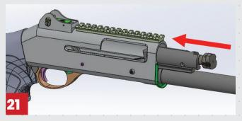
21- Insert the bolt by sliding it along the rails of the receiver. (fig. 21)
