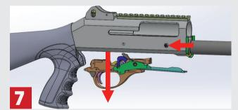
7- Push and hold down the bolt release button, then pull the fire control group out of the bottom of the receiver. (fig. 7)
