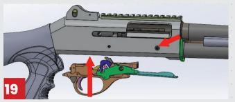
19- While holding the bolt release button, insert the fire control group into the shotgun and ensure the hole in the fire control group is lined up with the hole in the receiver. (fig. 19)
