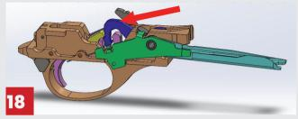
18- Take the fire control group and make sure the hammer is cocked with the safety on. (fig. 18)
