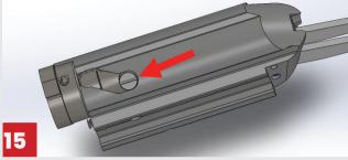
15- Insert the locking head retaining pin so that the line in the head of the pin is parallel with the bolt to allow a clear path for the firing pin. (fig. 15)
