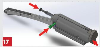
17- While holding the locking head into the bolt insert the firing pin and hold it flush with the back of the bolt. While holding the firing pin and locking head simultaneously, insert the firing pin retaining pin. (fig. 17)
